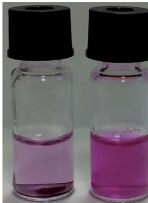
Fig. 4 Photograph of 1 (left vial) and QD-1 (right vial) in PBS buffer at pH 7.4. [ 1 ] = [ 2 ] = 0.187 mM.
